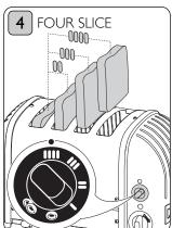
**4 slot model:** Rotate the 'selector switch' clockwise to the four slice indicator. All slots will heat up.
